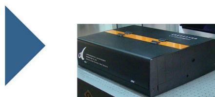
图2 全固态单频连续波绿光激光器(5瓦级输出) Figure 2 All-solid-state single-frequency continuous-wave green laser
